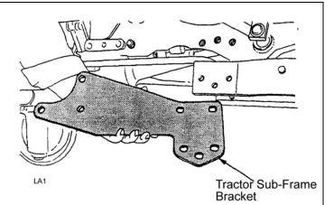
**Figure 1**. Remove Tractor Front Sub-Frame Brackets (B3200)
